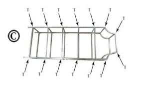
3.Screw the other frame with screws as illustrated C
